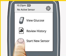
3 Hold the reader near the sensor to scan it. This starts your sensor. If sounds are turned on, the reader beeps when the sensor has been successfully activated. The sensor can be used to check your glucose after 60 minutes.
